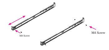
Mounting the rear ear bracket to rear side of rail. Adjust the rear ear bracket according to depth of your cabinet. If a screw hole is available, secure ear bracket to outer rail with a M4 screw. If only open slot is available, secure rear ear bracket with outer rail with screw. Do not tighten screw yet.
