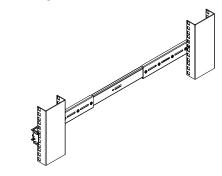
**6** Attaching center rail to right side of shelf. Make sure all 4 screw holes are aligned. Secure center rail to shelf with (4) M4 screws.
